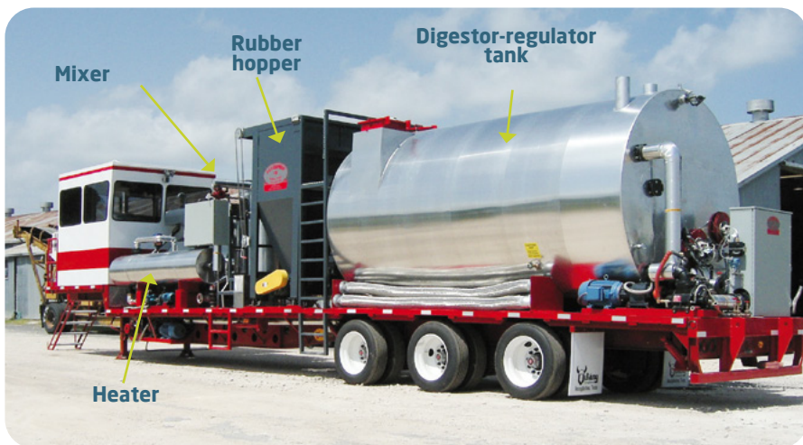
Figure 16. Manufacturing unit with mixer and digestion tank
