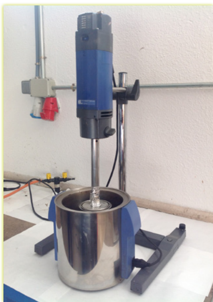
Figure 10. Setup of the basic laboratory equipment used to manufacture rubberised binders
