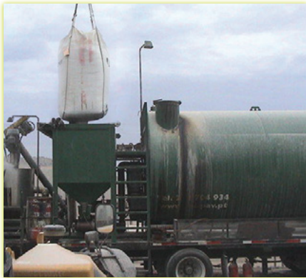
Figure 18. Detail of the loading of crumb rubber into the hoppers
