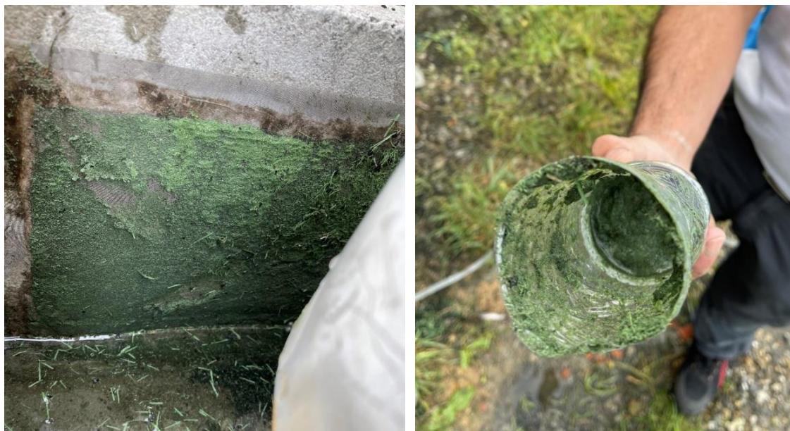
Image 12: Clogging of the filters of the general drainage manifold mainly due to the accumulation of fine particles of polyethylene fibres from the artificial turf.
